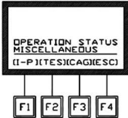
During the testing in our laboratory, the electronics is set for the I.R. cages. However, in case it is necessary to set it again, for example after replacing the batteries, etc., proceed as follows: from the main menu, depress the F1 (OPR) key (see previous display), followed by F3 (MIS) key.
