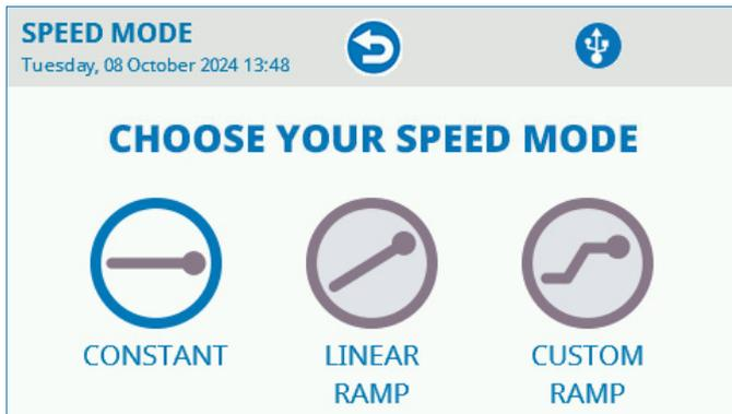
"Speed Mode" Menu: choose between Constant Speed Mode, Linear Ramp (increasing/decreasing speed) or Custom Ramp (upload a custom ramp directly via USB storage or LAN)
