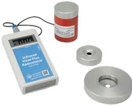
37300 - I.R. Heat-Flux Radiometer for Tail Flick and Plantar Test
