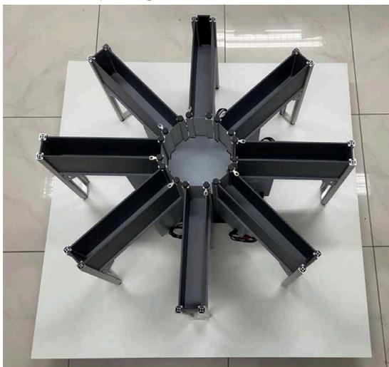
Regulate the two levelling feet at the external end of each arms to level the arms vs. the central arena plane; the space between the central arena and the arm floor (see from above) has to have the minimum space possible, which means the floor and the central arena plane needs to be at the same level.
