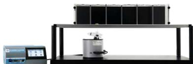
37550 - Dynamic Plantar Aesthesiometer - For Automated Mechanical Stimulation and Allodynia
