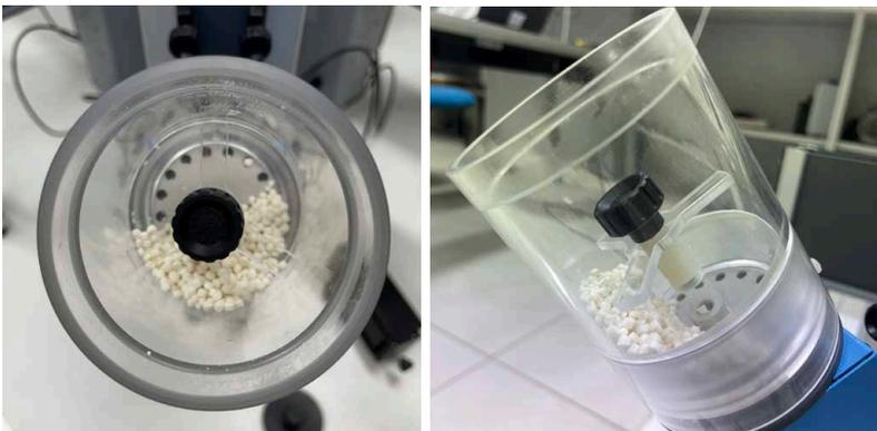
Do not press the separator down the tank, just gently place it inside.
