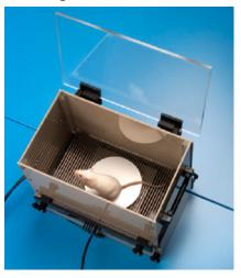
The detachable circuplatform, diam. 7cm, is positioned at the centre of the cage, on protruding stud fastened to the actuator, the mechanism which energizes the platform vibra-
