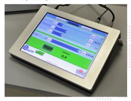
The Unit, incorporating a 12" touch-screen, manages the Passive Avoidance Test via the **40570-010** Software. Up to 4 cages can be connected to the same Controller.
