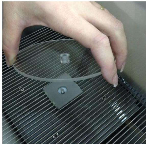
The Cage is provided with a **catch pan** which slides in, on two side rails, below the floor grid. The platform can be easily removed.
