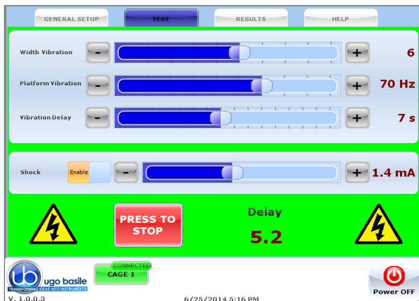
When the animal steps down from the platform, the operator stops the test, and the latency timer by depressing either the **“PRESS TO STOP”** button on the touch-screen, or the pedal switch.
