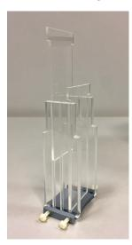
The set of accessories for mouse **35250-003** consists of two special tubes, with a 45x95(h)mm opening, connected by a metal bridge, whose width was minimized to 4cm.
