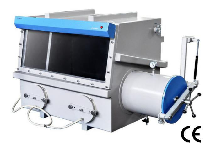
VGB-4A is a heavy duty stainless steel glove box equipped with airlock chamber, gauges, and vacuum flanges. This glove box can operate under vacuum to remove moisture and oxygen without expensive inert gas purging, It is an ideal tool for material and chemical researchers to process air sensitive materials and solutions.
