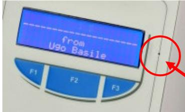
If the problem persists, charge the internal battery and reset the PAM manually by pressing with a needle into the small reset hole located to the right of the display.
