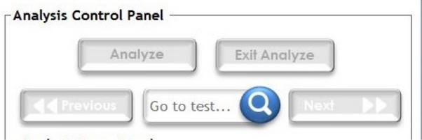
Once the experiment is over and the data transmitted from the device to the computer, push the button “**Analyze**” to open the folder where the .PAM files are saved and stored during the test.
