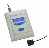
The P.A.M. (Pressure Application Measurement) device is an original tool designed for **measuring mechanical pain threshold on rodent joints**.
