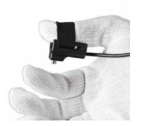
The PAM applies a quantifiable force for direct stimulation of the joint delivering an automatic readout of the animal response.
