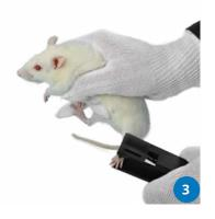
(1) Thumb force sensor to apply force to rat and mouse joints
