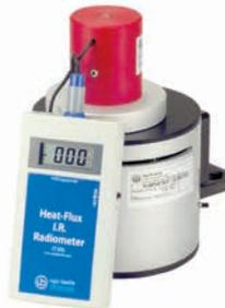
I.R. Heat-Flux Radiometer for Tail Flick and Plantar Test
