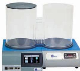
Thermal Place Preference (TPP Test) for Mice & Rats
