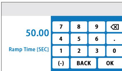
*The keyboard page to input the force rate in seconds*
