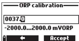
7. Once the reading has stabilized, the countdown timer will count down until the display shows the “Ready” message. Press **Confirm** to accept the calibration point.
