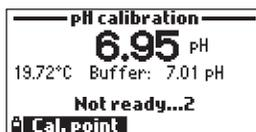
7. If necessary, press **Cal. point** to select the correct buffer. To use a custom buffer, press **Custom**. A text box window will appear. Use the keypad to enter the value of the buffer (0.00 to 14.00 pH) at the current temperature. Press **Accept** to confirm the buffer value.
