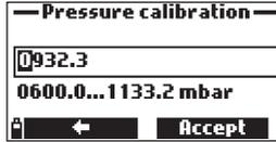
4. The stability timer will count down until the display shows the “Ready” message. Press **Confirm** to store the calibration point.
