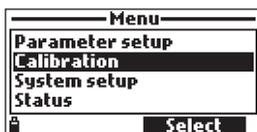
All calibration data is stored in the non volatile probe memory, allowing probes to be connected to different meters without recalibration.
