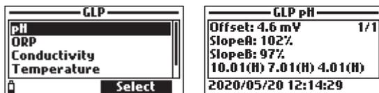
*Notes: A "C" label near the buffer value indicates a custom point, while an "H" indicates a Hanna Instruments standard buffer value. If a quick calibration was performed, buffer values are replaced with "Quick calibration" indication.*
