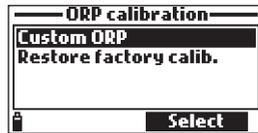
The calibration should be performed at temperatures between 20-26 °C.
