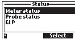
Use the arrow keys to navigate through the meter status information. Press **ESC** key to return to the “Status” menu.
