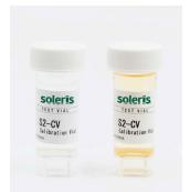
Pictured: Acceptable S2-CV vial (left) and unacceptable vial (right).
