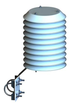
The **WxRS-150** provides protection for temperature and humidity sensors by shielding them from external air. The sensors are doubly protected to minimize the impact of weather phenomena such as radiation and precipitation. It ensures that there is no temperature variation caused by aerosols or raindrops. (The fan is optional.)
