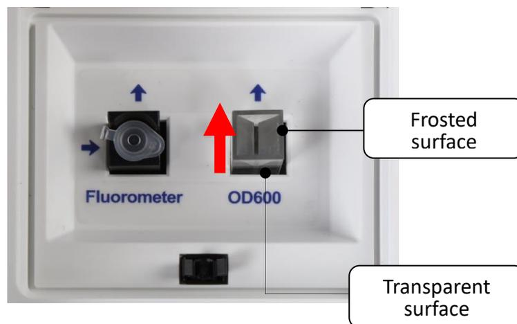
**Fig. 7 OD600 & Fluorometer Port**
