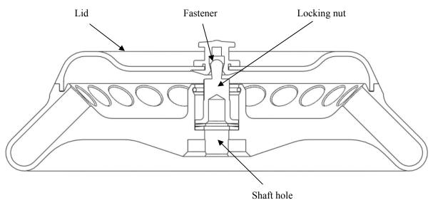
Figure 11-1 The rotor structure
