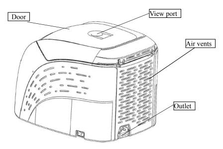
Figure 5.2 Rear view of the centrifuge
