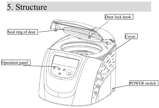
Figure 5.1 Front view of the centrifuge
