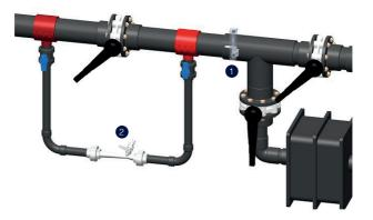
The ideal installation of the inlet kit is ① with a 1/2" tap after the filter and heater. The entire inlet kit: fittings, isolation valve and flow meter are supplied with the dosing unit.
