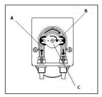
The principle of operation of the peristaltic pumps is based on pressure and subsequent release of the inner tube (A) by the roller (B) mounted on the roller-holder (C), which is driven by the motor.
