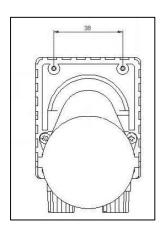
The pump should be installed on a vertical support, using the fixing points shown in the figure, in such a way that the pump always remains in a vertical position ( $\pm$  15°).
