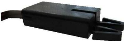
**Important note:** In case you need to remove the cable, use a screwdriver to bend the clips and push out the connector. Carry out this operation very carefully, because the connector clips may easily break.
