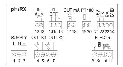
For correct electrical connections always refer to the rear panel pad printing, specific for each model. The above figure represents the pH/RX model version.
