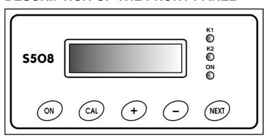
ON key Enable / disable all outputs (relays, pump magnet, mA output)
