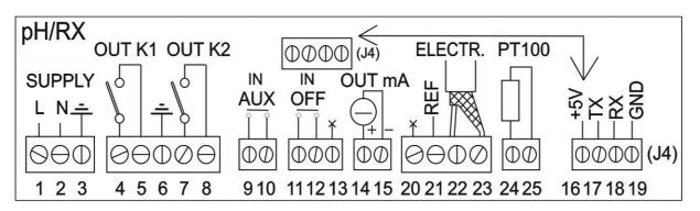
For correct electrical connections always refer to the rear panel pad printing, specific for each model. The above figure represents the pH/RX model version.
