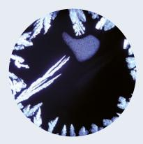
In this temperature range it is difficult to know, without visual observation, whether the system is controlling at the dew point, at the frost point, or somewhere in between. Since these states occur at different mirror temperatures for gas of the same water vapor content, it is important to determine which it is. Errors resulting from this problem can be up to 3°C.
