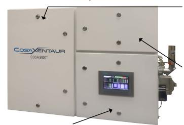
The Sample Conditioning Enclosure contains sample conditioning and the gas mixing system. Components in this compartment are intrinsically safe. The gas mixing compartment is heated to avoid condensation of heavier gas constituents.
