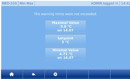
The temperature memory records the maximum and minimum temperature values reached during operation.
