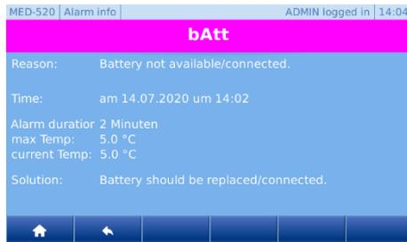
If a function of the unit is faulty or defective, an alarm is triggered. Every alarm is displayed visually as well as acoustically.
