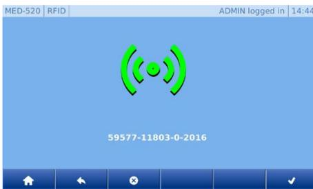
6. Hold the RFID transponder in front of the RFID sensor until you hear the confirmation tone and the symbol on the screen lights up green. The number of the RFID transponder also appears.
