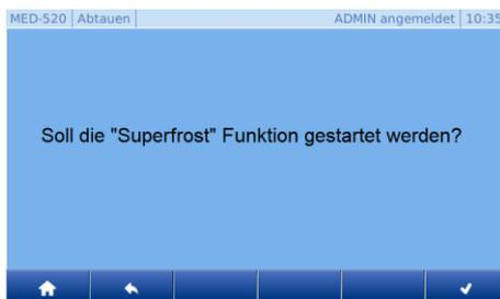
By activating the "Superfrost" function, the refrigerator reaches the lowest possible temperature inside.
