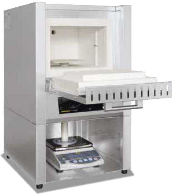
Weighing furnace L 9/11/SW with flap door
