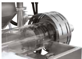
Flange with heat radiation protection insert (gas supply system 15)
