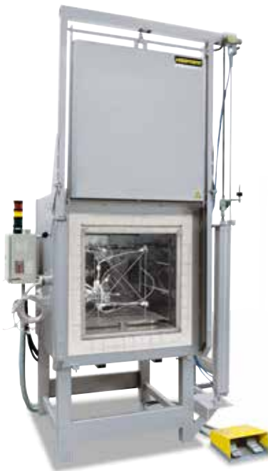
Holding frame for measurement of temperature uniformity
