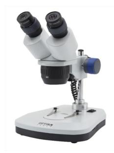
Stereomicroscope, with pillar stand, 20x-40x, with rechargeable battery
