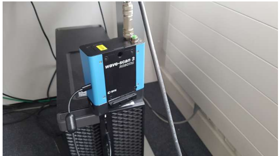
Illustration 14: Sample test setup for wave-scan 3 ROBOTIC
