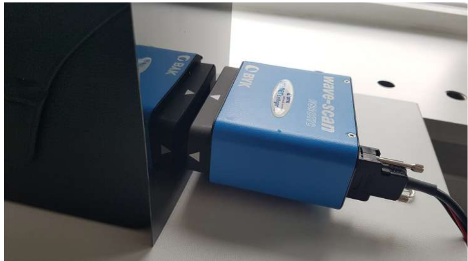
Illustration 151: BYK-Gardner wave-scan ROBOTIC - Simulator setup
