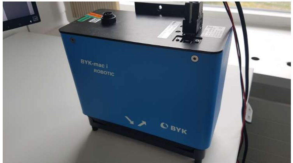
Illustration 46: BYK-mac-Device on calibration tile
