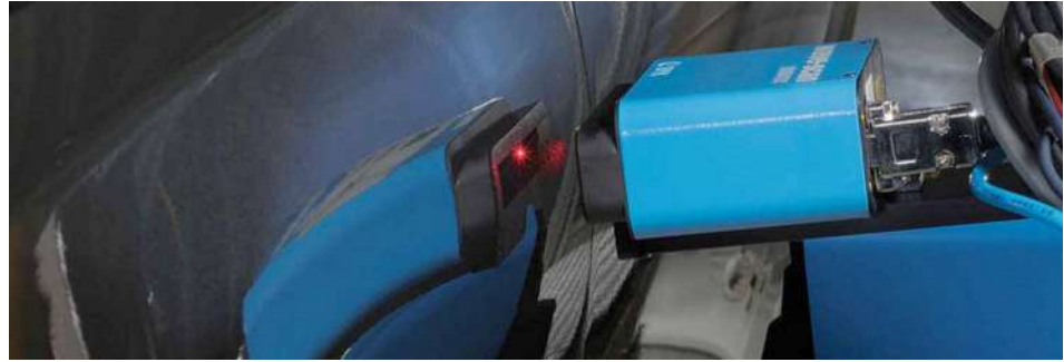
Illustration 2: Instrument wave-scan ROBOTIC on robot arm
