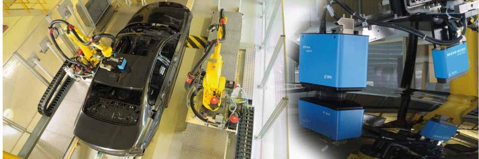
*Illustration 22: Robot cell with two robots / Robot arm with two instruments*
