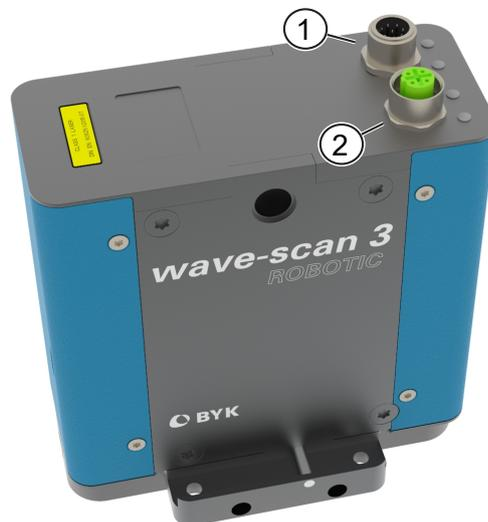
*Illustration 4:* Interface connectors of wave-scan 3 ROBOTIC
