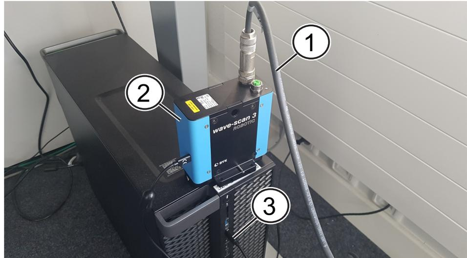
Illustration 18: Cabling for connection test
