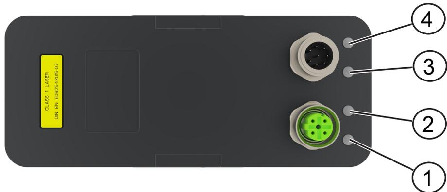
*Illustration 5: Status LEDs of wave-scan 3 ROBOTIC*
