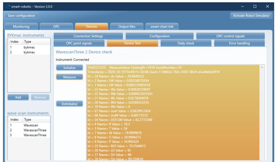
Illustration 21: Device test in smart-robotic
