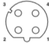
Illustration 10: Pin assignment M12, 4-pin, D-coded, view socket side
