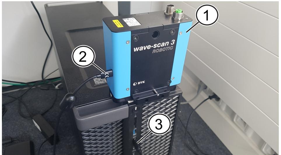
Illustration 16: Cabling for USB driver installation
