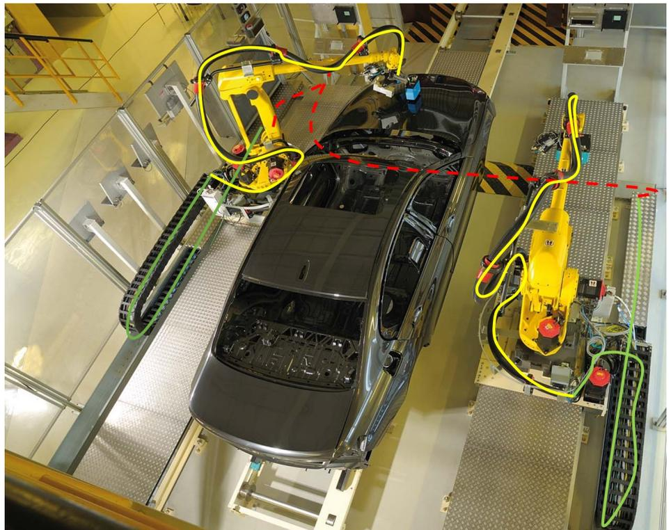
*Illustration 6: Example cabling in a robot cell*
