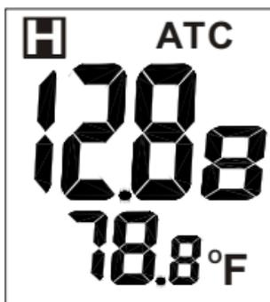
1. During measurement, press **HOLD** to freeze the reading on the display. "H" appears at the top of the LCD and the pH decimal point stops flashing.
