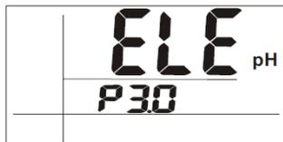
4. Press **MN/MX/AV** to enter P3.1, the LCD displays one of four available slope values; P3.1, P3.2, P3.3, P3.4. If the value is less than 75% or more than 115%, change the probe immediately.
