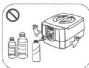
Do not fill the tank with abrasives or corrosive chemicals.
