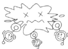
Bubbles are imploded constantly under the action of ultrasonic to impact the surface of the item.
