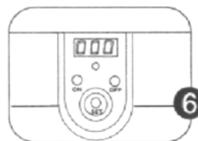
When reach the time of "00" the unit will auto stop, the red light will turn off. If another cleaning is needed, just repeat the above steps. During cleaning, if you want to stop, just press "OFF" button. Press "NO" button again, the unit will implement the remainder program to continue the cleaning. Furthermore, you can press "SET" button to renew working cycle.
