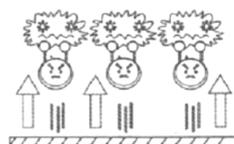
The impact splits up the dirt into many granules and separates them from the surface of the item, the granules then come into water.
