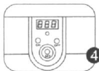
Press "SET" button to choose working cycle freely. When the unit is electrified, 180s is displayed automatically, it is the most common-used working cycle. Every time when press "SET" button, the 5 optional working cycles from →280S→380S→480S→90S will be displayed on the screen.
