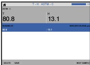
After the measurement is finished, the results appear in the display. The progress bar right in the header and the number of readings are incremented, e.g. 1/3 means that the first of 3 readings per sample is performed.
