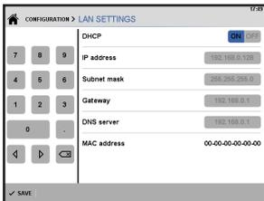
In the delivery configuration the DHCP switch is set to “ON”, which means that the DHCP server provides all necessary information to your instrument.
