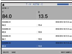
If you continue with further measurements, the results of each single measurement are listed. The average values are displayed in bold letters above the single readings.
