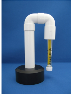
Figure 2: Tube and head adaptor assembly
