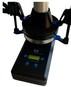
Switch on the barometer and wait for a short period for the air pressure to be displayed. The reading is in millibars; record the atmospheric pressure.
