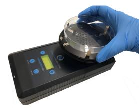
If calibrating a MicroBio model of sampler, then the MicroBio adapter ring must be fitted onto the MicroBio sampling head before fitting the calibration rig.
