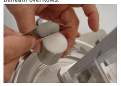
Now level off the powder using a flat edge scraper. Re-weigh the cup and calculate the weight of the collected
