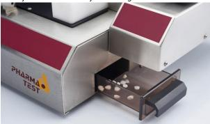
Once the test is finished and the sample is broken, the sample dish moves backwards to drop the sample fragments into the removable waste container. The results are immediately displayed and may be printed on a connected printer. The print-out includes each individual result as well as product information, date, time, user, instrument serial number and statistics.
