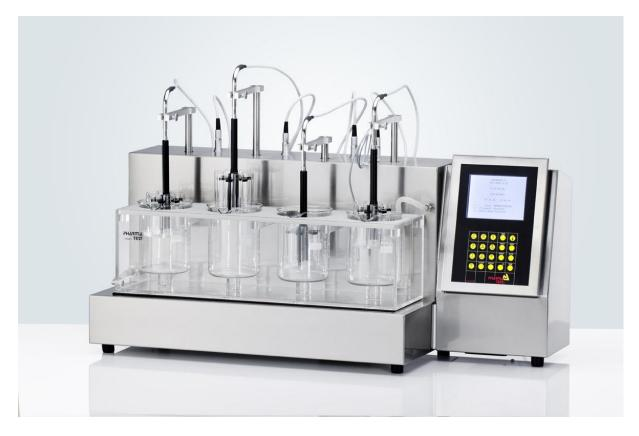
A large 320x240 pixel LCD screen and an alpha-numerical keyboard are used to edit product and test information, such as the target disintegration time for each station and the bath and media temperatures. Up to 16 different testing methods can be filed in the instrument's memory.
