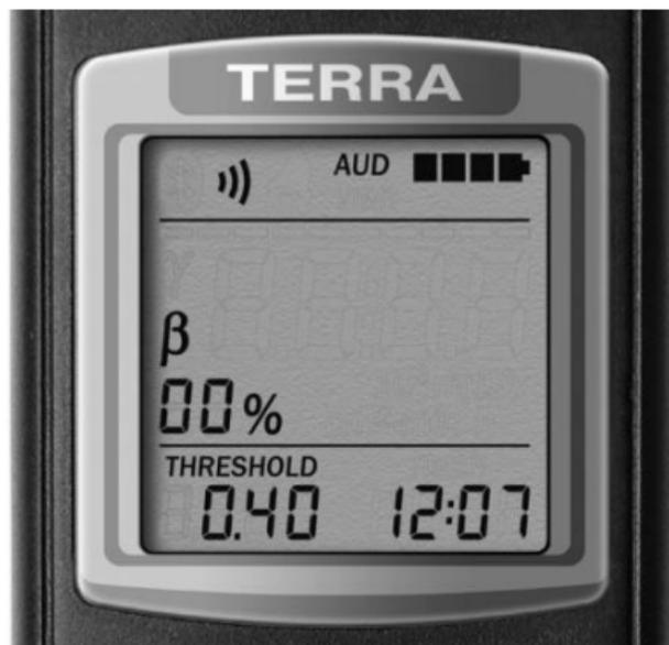
Figure 15 – LCD of the dosimeter
