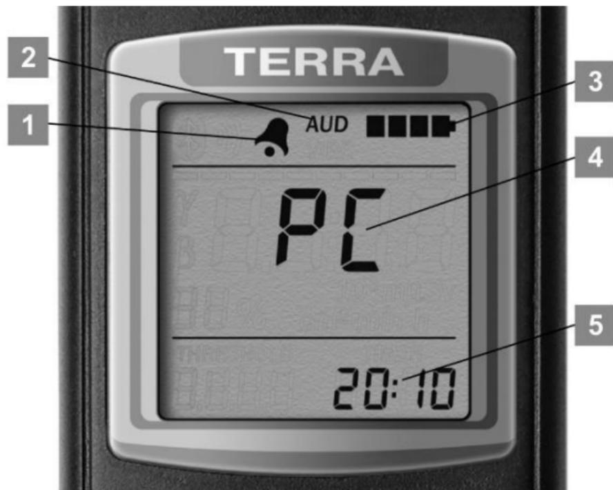
Figure 27 – LCD of the dosimeter
