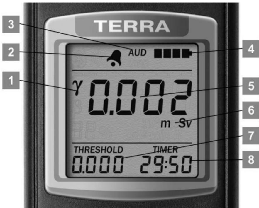
Figure 11 – LCD of the dosimeter
