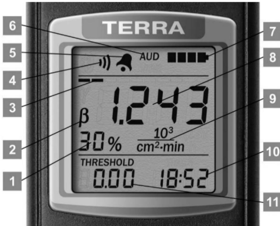
Figure 14 – LCD of the dosimeter
