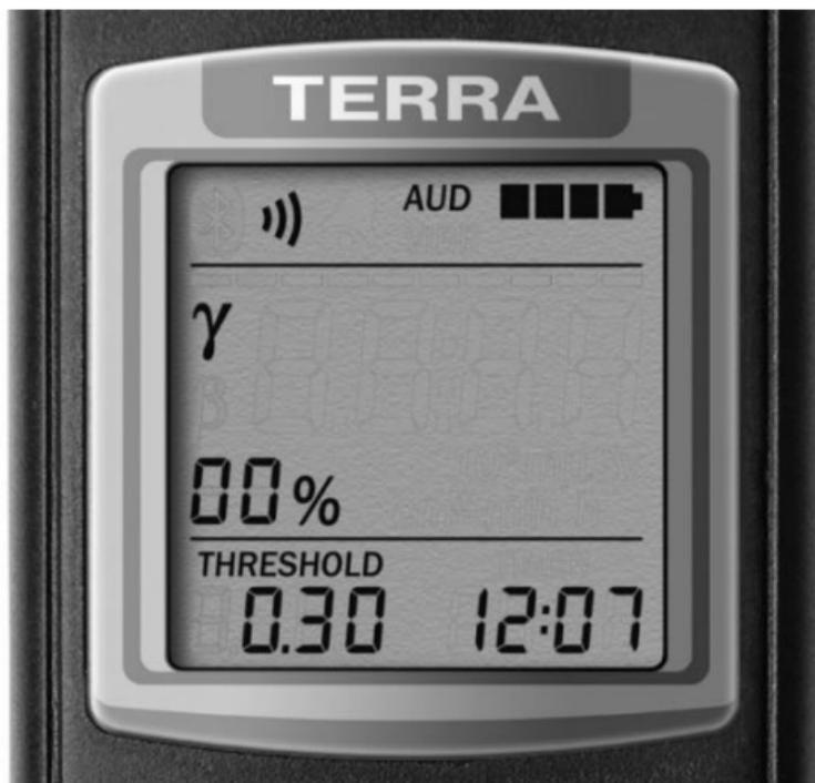
Figure 4 – LCD of the dosimeter
