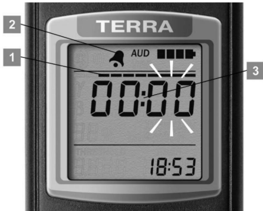
Figure 26 – LCD of the dosimeter
