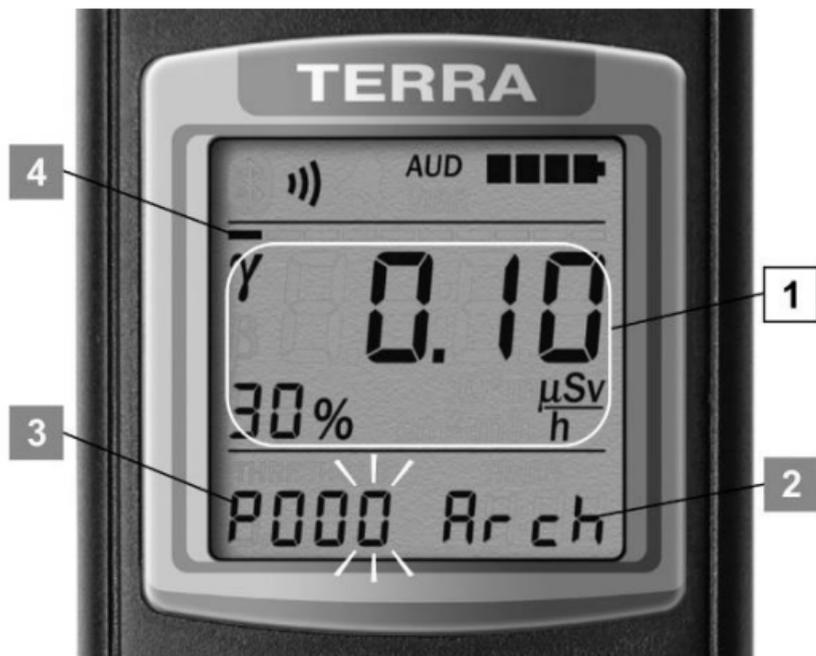
Figure 10 – LCD of the dosimeter
