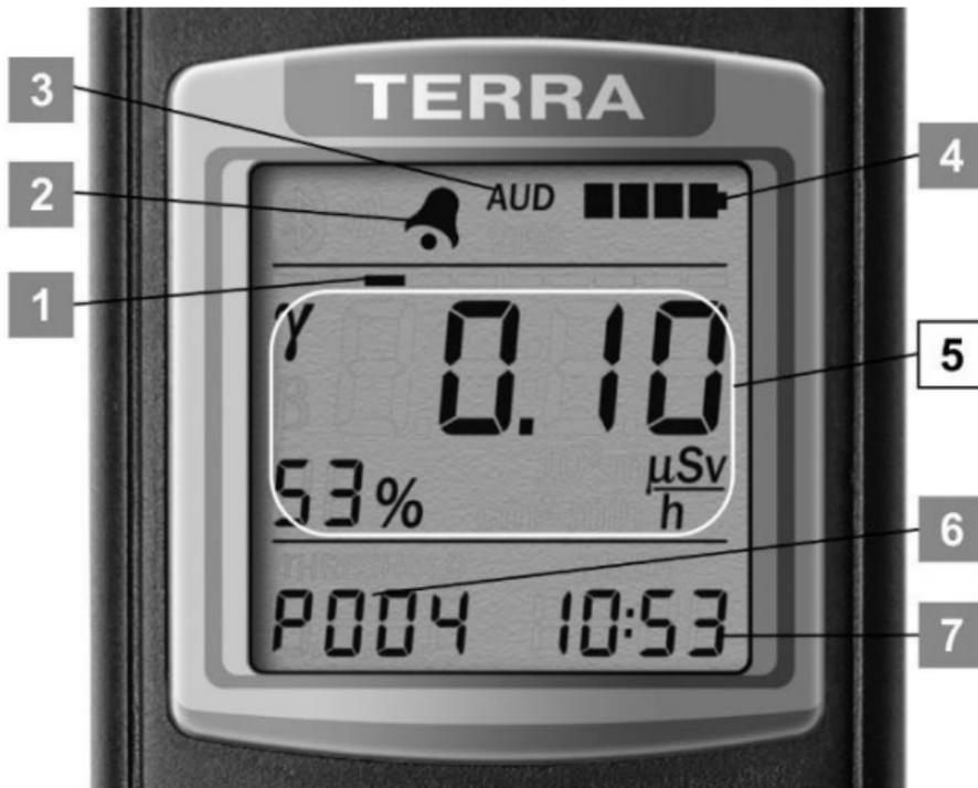
Figure 30 – LCD of the dosimeter
