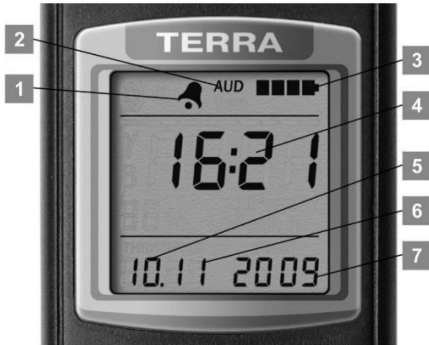
Figure 21 – LCD of the dosimeter
