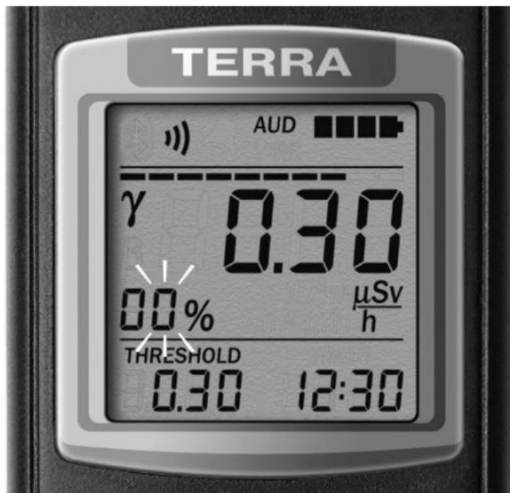
Figure 8 – LCD of the dosimeter
