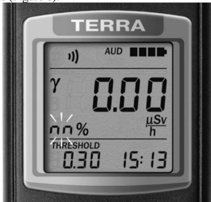
Figure 6 – LCD of the dosimeter (measurement restart)
