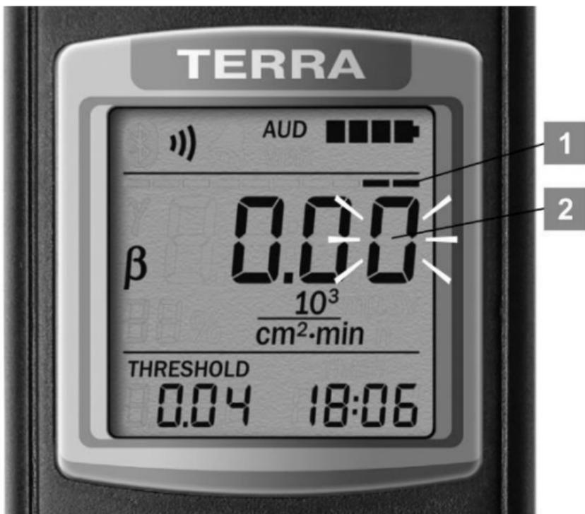
Figure 18 – LCD of the dosimeter
