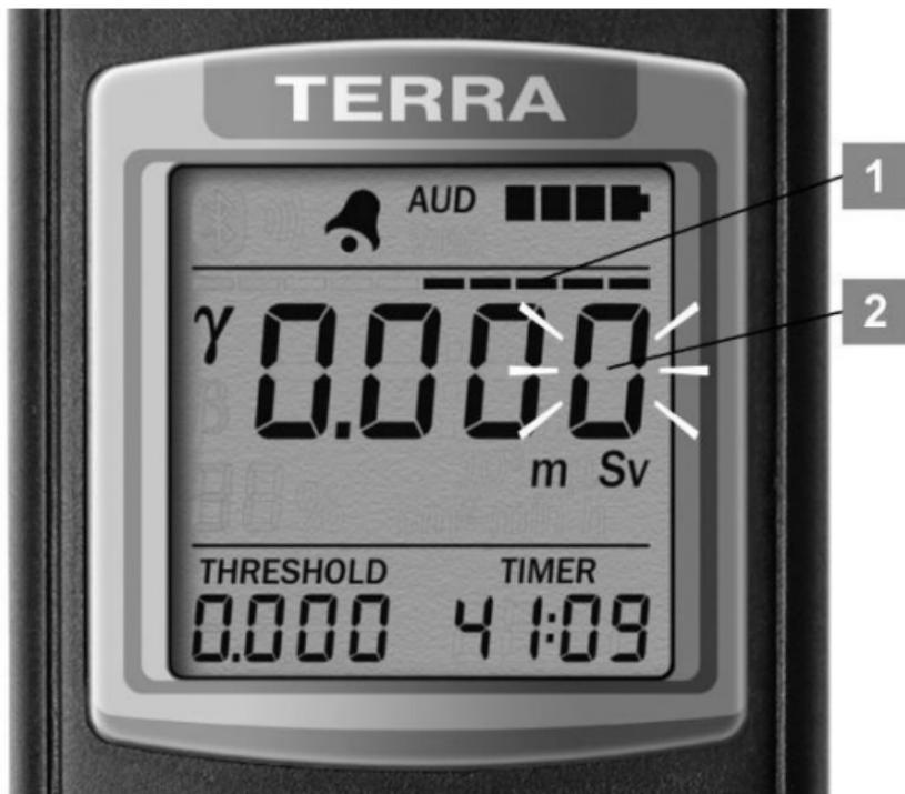
Figure 12 – LCD of the dosimeter
