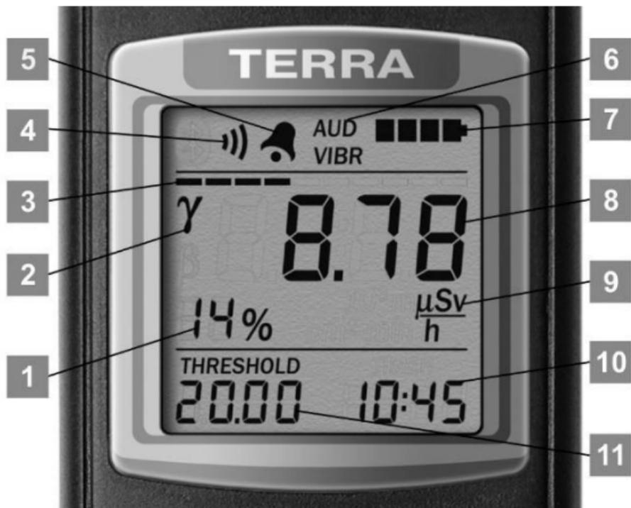
Figure 3 – LCD of the dosimeter
