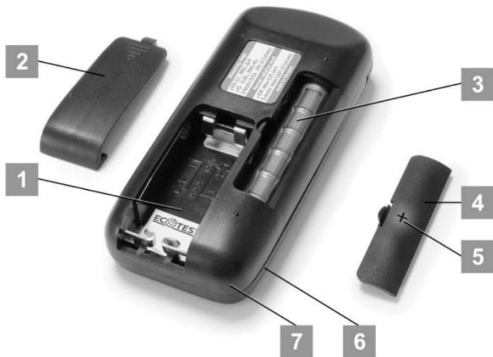
Figure 2 - External view of the dosimeter (bottom view)
