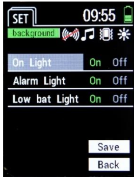
Figure 22 – Setting light signals
