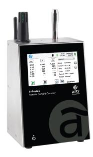
The Airy Technology® B306 and B506 Remote Particle Counters measure 0.3 or 0.5 to 25.0 µm with a flow rate of 0.1 CFM (2.83 LPM). Easy to configure, these instruments display up to 6 user-selectable size channels as well as (optional) temperature and relative humidity. View data or export to Instrument Management Software (IMS). Airy Technology® counters can be controlled and monitored remotely via web browser.
