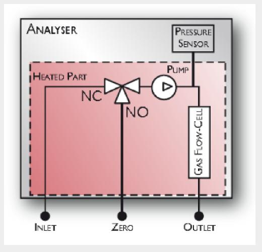
Three gas connections are available on the rear panel of the analyser:
