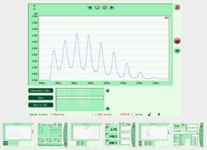
A colour touch screen display interface allows the user to easily navigate through a number of screens that are used to set and check all of the operating conditions of the instrument. A protective film limits the risk to damage the surface of the touch screen, especially against solvent and corrosive liquid.
