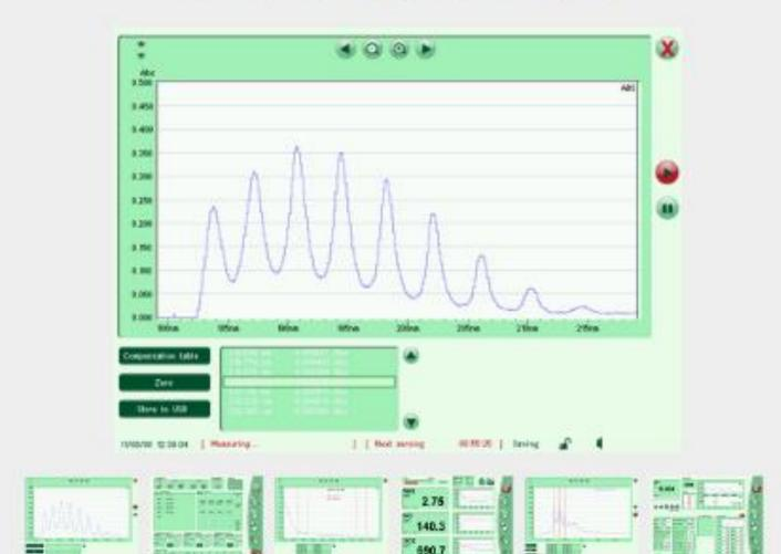
A colour touch screen display interface allows the user to easily navigate through a number of screens that are used to set and check all of the operating conditions of the instrument. A protective film limits the risk to damage the surface of the touch screen, especially against solvent and corrosive liquid.
